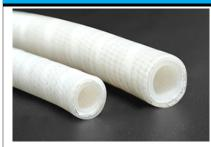
**HiPoWrap** is Platinum cured Silicone hose reinforced with SS 316L Helical wire and 2-3 layers of polyester fabric wrapping. **HiPoWrap** is having multiple layers of high quality polyester fabric to enhance burst Pressure rating. The product is suitable for high pressurized Steam transfer application in pharmaceutical and biotech.
