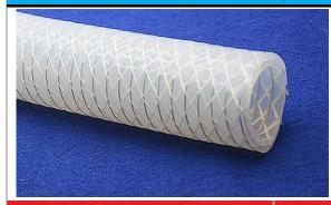
**HiPoTorr** is Platinum cured Silicone hose reinforced with SS 316L Helical wire and polyester braiding having better flexibility with high pressure resistance. **HiPoTorr** is having high burst pressure rating along with high vacuum resistance compare to **HiPoVacc**. The product is suitable in pressurized fluid transfer application.
