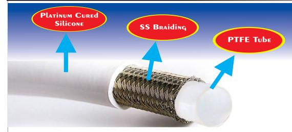
**HiPoTeff** is PTFE tubing covered with SS 304 braid reinforcement having outer layer of Platinum grade silicone. **HiPoTeff** is having capacity to withstand high pressure along with greater chemical resistance. The product is having ultra smooth bore which enhances superior flow properties & least adhesion to particulates. The outer layer of Silicone cover acts as insulation to high temperature and keeps outer surfaces dust free.
